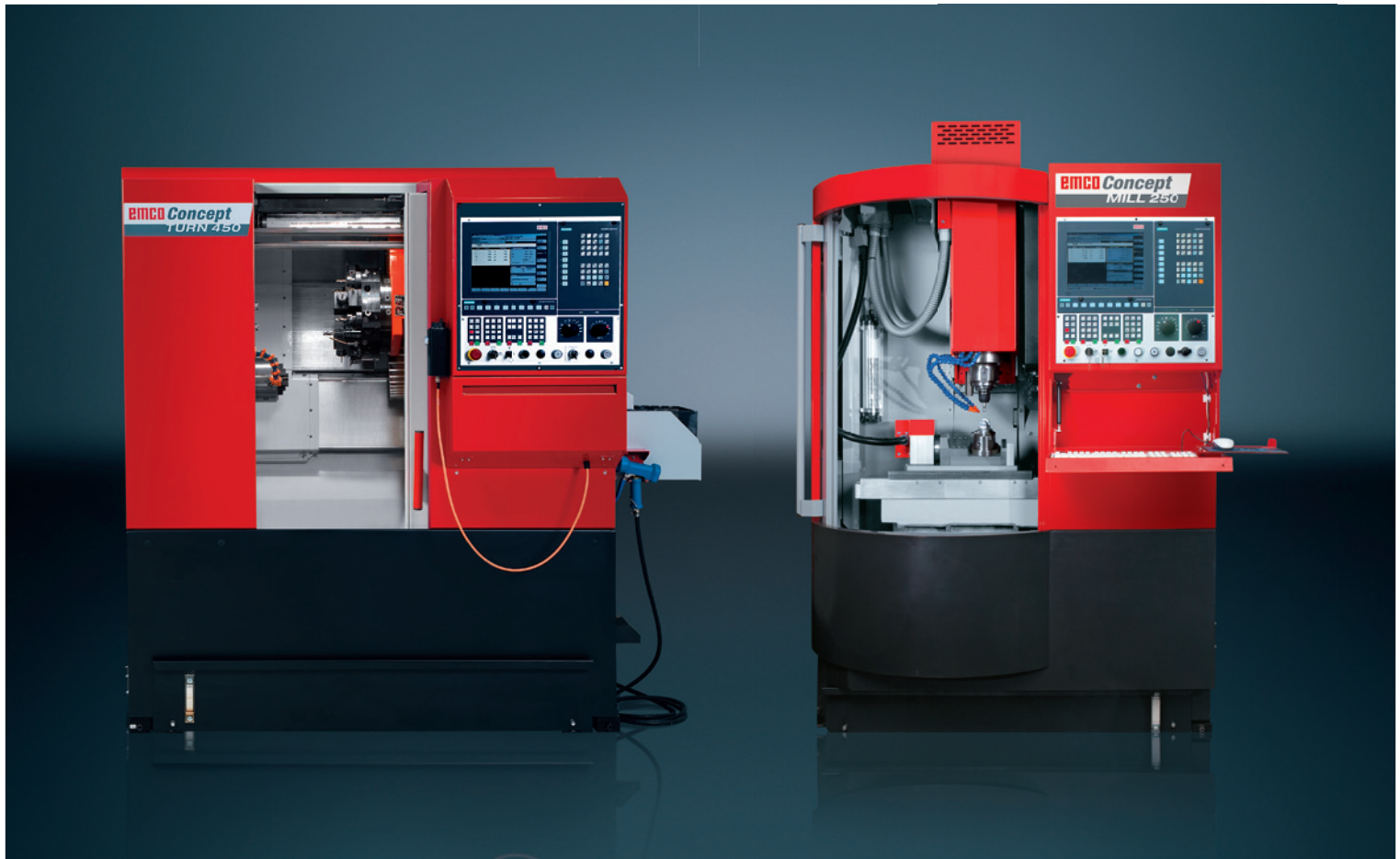
Concept Turn 450 and Concept Mill 250 used in the practical workshops for mechatronics and conventional cutting
