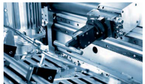
Chain feeding system with V-supports for preformed shaft parts of various shapes.
