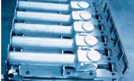
6-station pallet attachment for articulated brackets
