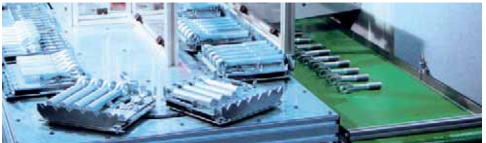
20-station pallet magazine with customer-specific pallets
