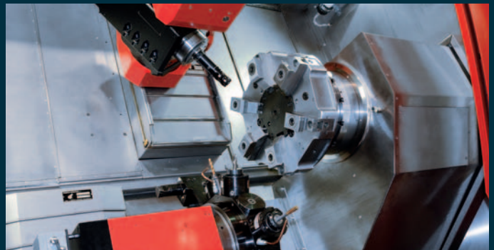
Counter spindle view with 6-position jaw chuck Ø 500 mm. The upper turret is replaced by a 21 kW liquid-cooled milling spindle in the B axis version. The B axis travel range is 205°. This is infinitely variable with 0.001° resolution. In addition, the B axis can be clamped in any position with 5° indexing.
