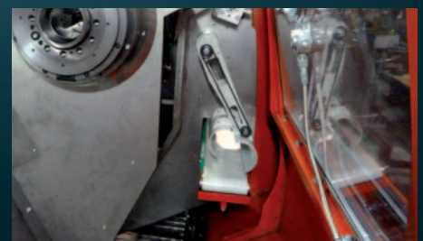
Parts catcher with conveyor: Finished parts are ejected with a coolant fed part ejector into the parts catcher and transferred with a conveyor to a storage area.
