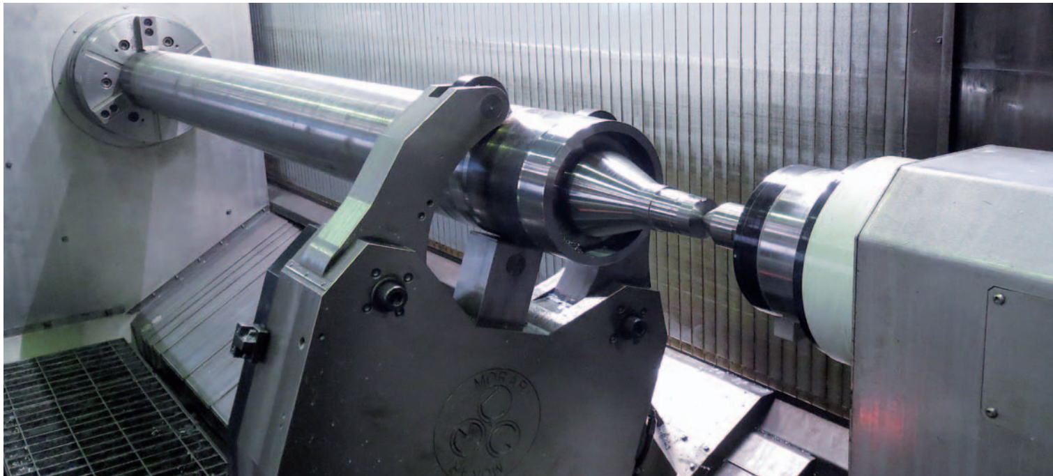
Foil rolls with a diameter of 350 x 3800 mm supported by the steady rest and tailstock
