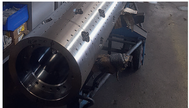
Some rolls require hundredfold drilling and milling with very narrow tolerances
