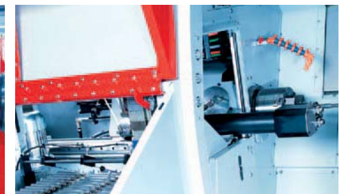
Fully automatic shaft loading. Feed-in via a conveyor belt, removal via the finished parts pick-up device
