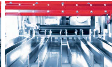
Multiple infeed chutes for loading rotationally-symmetrical blanks; the length of the blanks determines the number of infeed chutes.
