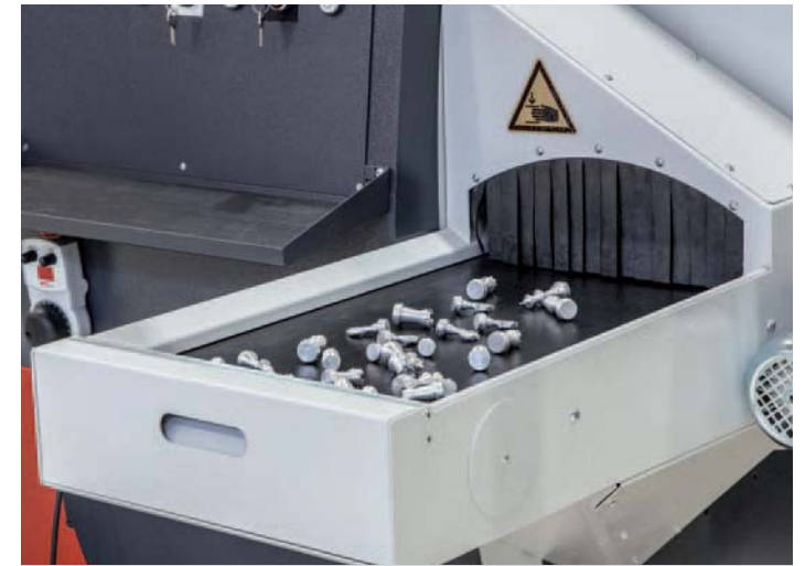
Finished parts conveyor. The parts catcher deposits the finished parts on an accumulating conveyor with a usable storage area of 340 x 750 mm.
