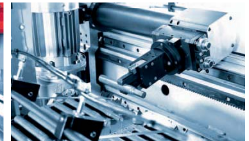
Timed conveyor system with V-supports for preformed shaft parts of various shapes.
