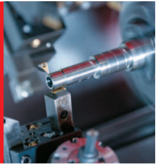
Simultaneous turning work is possible using both turrets on the main or counter spindle.
