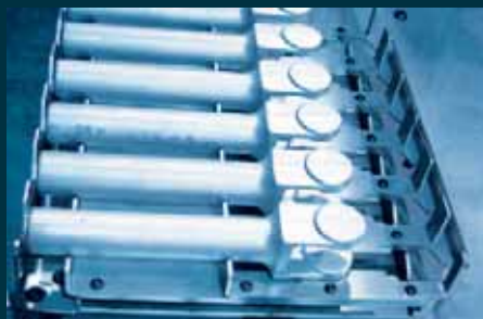
6-station pallet attachment for articulated brackets
