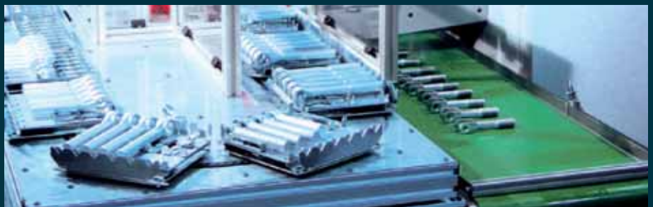
20-station pallet magazine with customer-specific pallets
