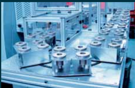
4-station pallet attachment for valve caps
