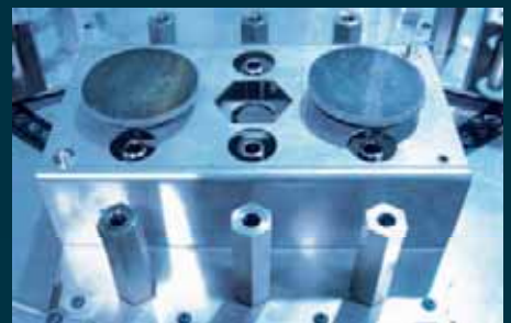
Multi-pallet attachment for a family of parts
