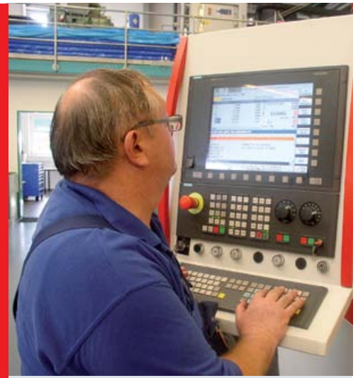
Pivotable and extendible control unit for optimum ergonomics for programming and running the machine.
