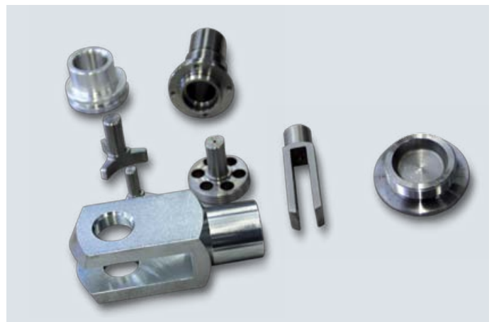
Examples of work pieces, made with the HYPERTURN 65-TRIPLETURN
