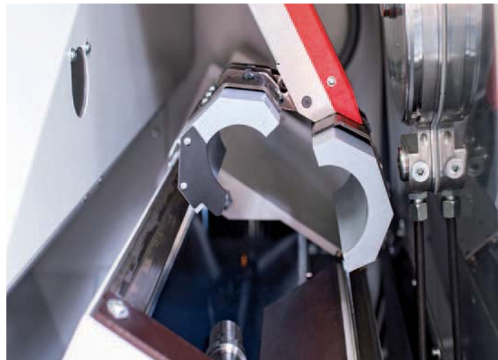
Parts catcher. The HYPERTURN 65's electro-pneumatic parts catcher is controlled using M functions. When needed, it traverses to the front of the work area and pivots to the spindle center. The finished part is removed from the clamping device and transferred to the catcher tray. The parts catcher then moves back to its initial position and the part is tipped onto a conveyor belt.
