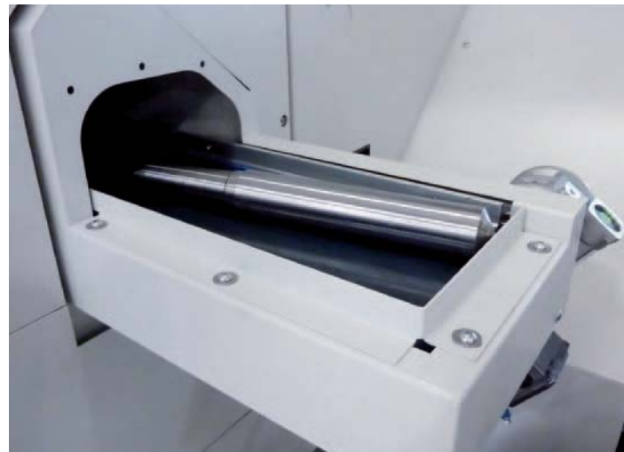
Finished part conveyor belt. On the conveyor belt within the machine casing, arranged lengthwise, with a storage surface of 1400 x 180 mm, the work pieces are put down damage free.
