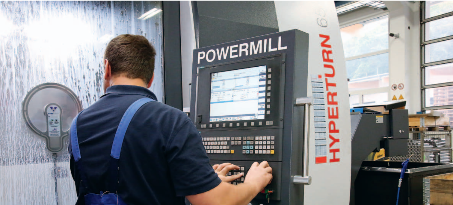
The Hyperturn 65 Powermill scores with user-friendly ergonomics and good workspace accessibility. A very large window provides an unrestricted view – the tool magazine and control are within the operator’s immediate reach.
