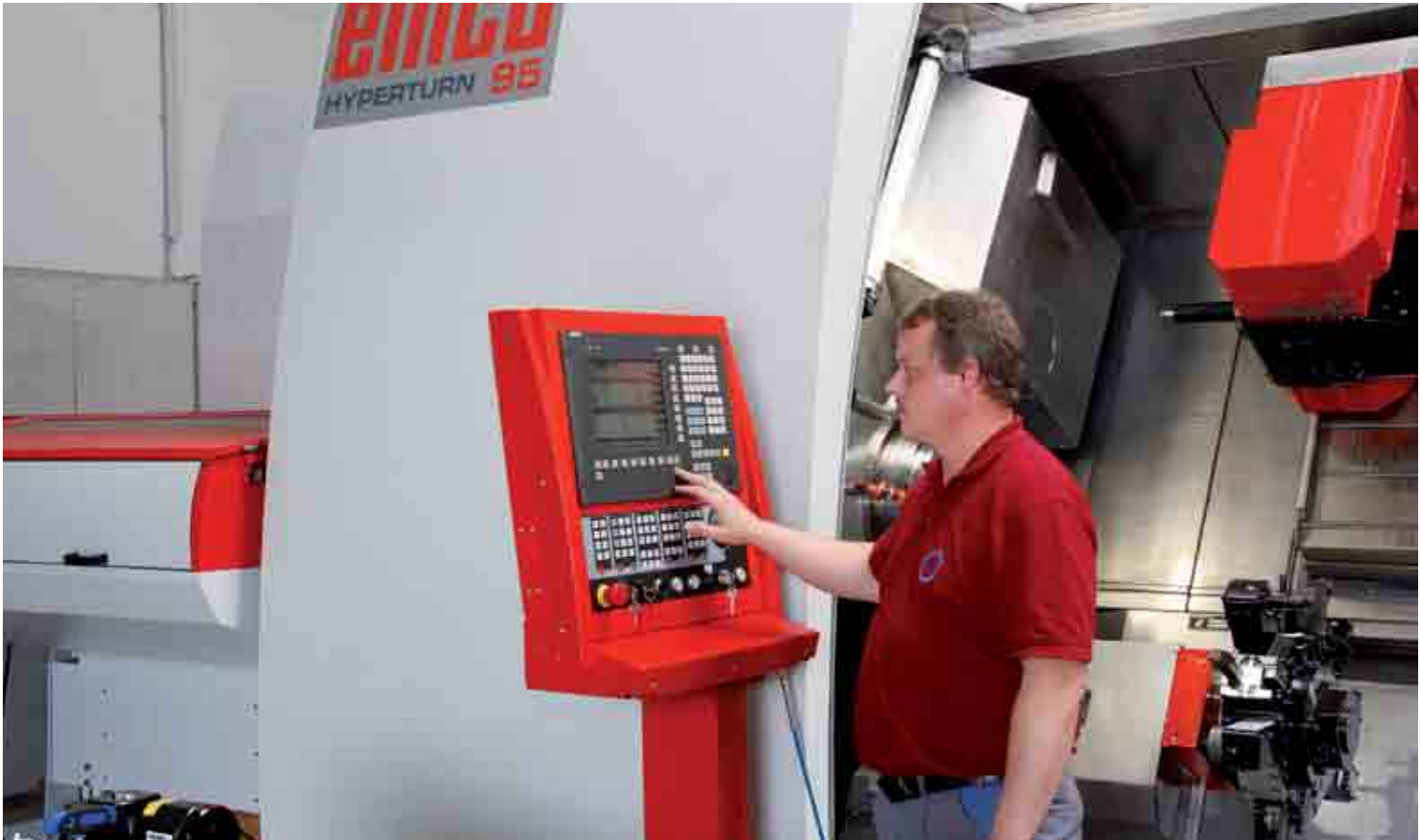
At MKE, programming tasks are performed with the ESPRIT CAM system, and also directly at the machine using the Sinumerik 840D-sl by Siemens. (note: pictured – Andreas Schramel, CNC Machinist)
