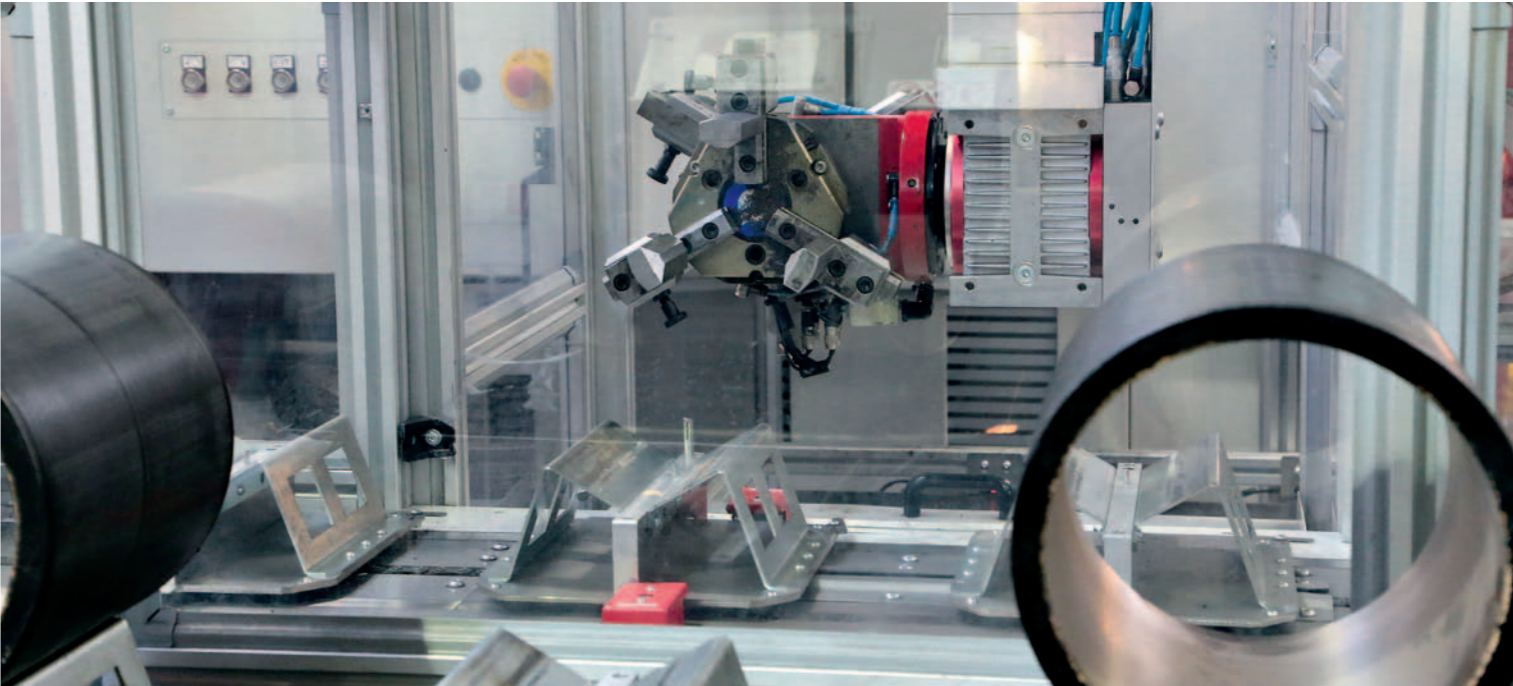
The gantry loader is equipped with a three-jaw gripper on either side for inside and outside hold. It can move workpieces weighing up to 40 kg at speeds of up to 120 m/min.
