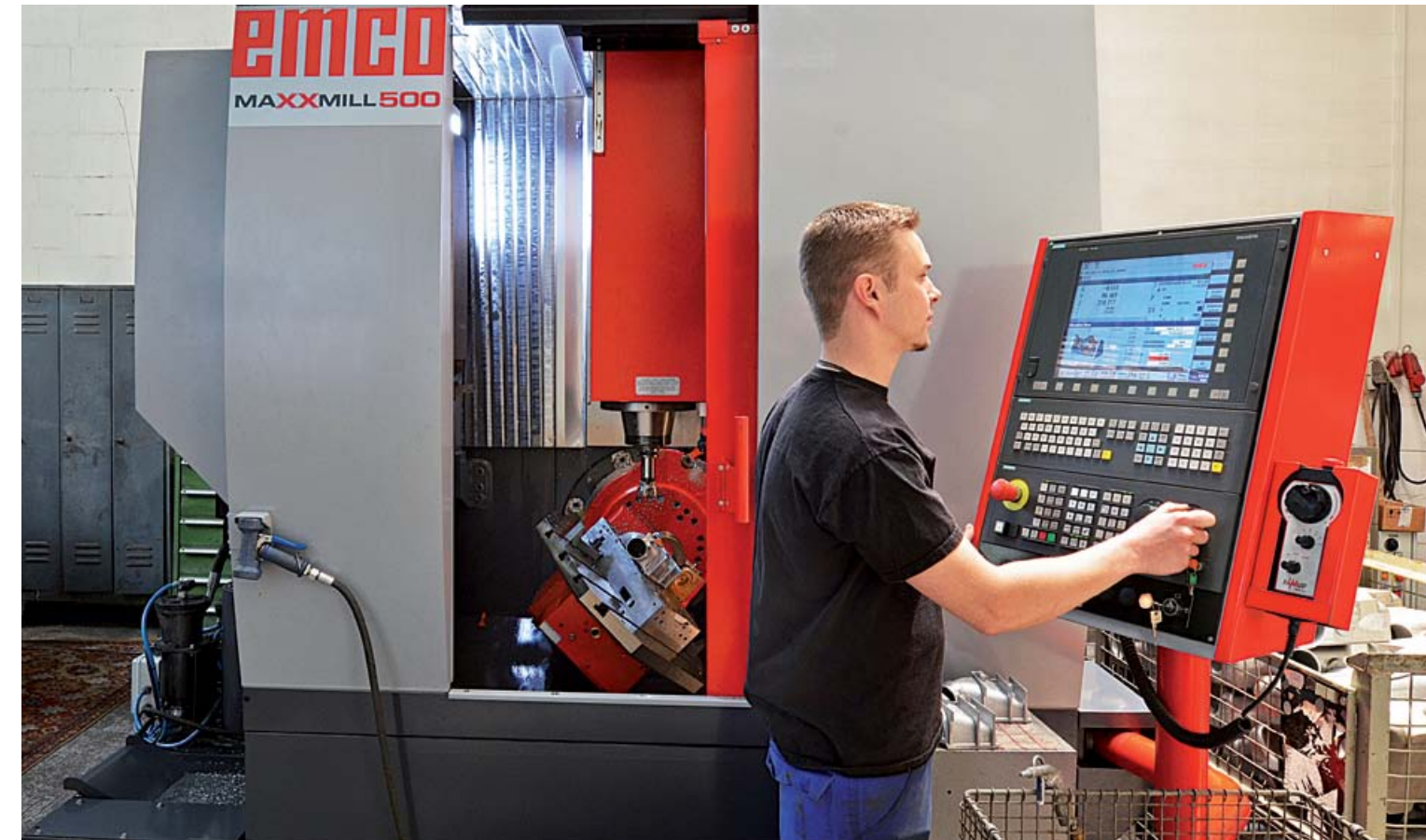
Maxxmill 500: vertical machining center for 5-axis machining
