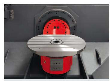
**Swivel-rotary table.** The swivel-rotary table has a large clamping area of  $750 \times 600$  mm ( $29.5 \times 23.6$ ") and can bear loads of up to 300 kg (661.3 lb). This makes it possible to simply machine workpieces with an edge size of  $530 \times 530 \times 417$  mm ( $20.8 \times 20.8 \times 16.4$ "). The special shape of the table allows the spindles to move closer to the table center.
