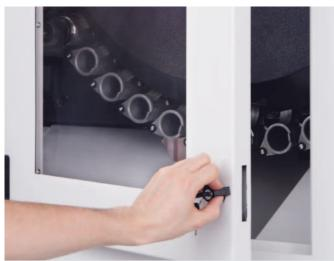
**Tool changer.** The tool changer is a drum magazine for 30 tools. A tool magazine with 40 or 60 tool stations is as option available. The tools are managed according to the variable tool stationcoding principle (random), which means that tools are always deposited in the first free magazine station for time reasons.
