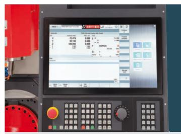
The Sinumerik 840D sl incl. Shopmil. The Sinumerik 840D sl incl. Shopmill is a universal and flexible CNC system and offers free contour programming, moving cycles for complex contours, fast reference point setting with touch probe systems, tilting the working plane, cylindrical surface machining, 3-D tool compensation, fast execution through short block processing times.
