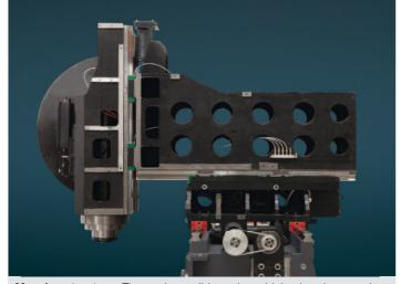
**Massive structure.** The carriage, slide and machining head are made of cast iron for maximum stability and best workpiece finishing. Cast components optimized by means of FEM analysis, which means that these components are lightweight and stable at the same time.
