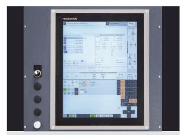
**Heidenhain TNC 620.** The TNC 620 is a compact, adaptable control for up to five controlled axes. With its flexible operating concept - workshoporiented programmability in the HEIDENHAIN plain text dialog or external programming – and its range of services, it is perfectly suited for EMCO milling centers.
