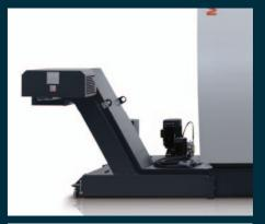
**Hinge type conveyer:** The chip rinsing system washes chips into the hinge type conveyer, which then automatically transports the chips from the machine into the customer provided container.
