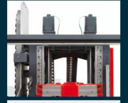
**Z-axis travel:** In order to attain precision Z-axis rapid travel at speeds of 40 m/min, and due to its large mass, this axis is powered by two ball screw drives and two motors in a master-slave configuration.
