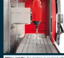
**Milling spindle:** The machine is equipped with a liquid cooled motor spindle with compelling performance specs. At spindle speeds of 15000 rpms, a power rating of 46 kW, and a torque of 170 Nm, the machine is also suited for heavy-duty machining. A motor spindle 18000 rpm is available with HSK A63.
