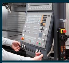
**Control unit:** The operator panel can travel, rotate and be adjusted in the direction of the work space. This ergonomic design provides ideal working conditions for the operator.
