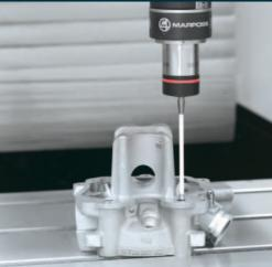
Measurement systems Tools measurements to reduce setup times during tool changes, as well as work piece measurements to verify dimensions or to find zero locations. The work piece measurement is radio.
