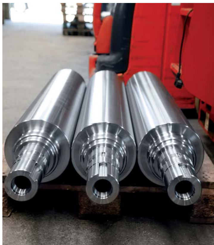
These drive shafts made of high-grade alloy steel with a diameter of 250 mm and a length of 2500 mm are completely processed using the Maxxturn 110.
