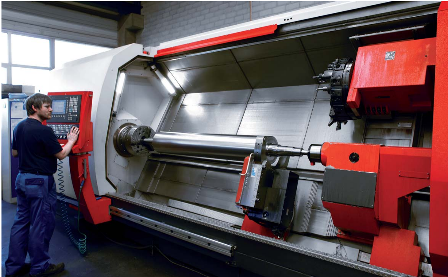
Embossing roller with a length of more than 2000 mm and a diameter of 300 mm processed with Maxxturn 110 x 3500 MY.
