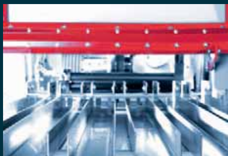
Multiple infeed chutes for loading rotationally-symmetrical blanks. The length of the blanks determines the number of infeed chutes.
