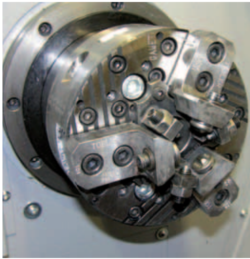
The chuck is customized to the dimensions of the raw parts.
