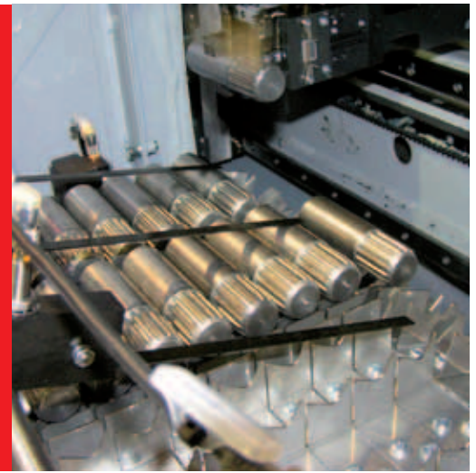
The finished driveshafts made of stainless steel connect the electronics with the mechanics in the pumps.
