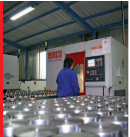
Quick loading through the spindle's direct pick-up of the raw material
