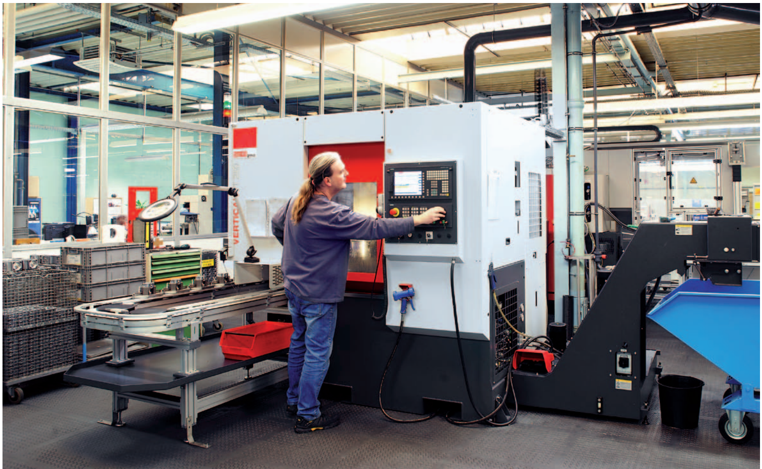
According to production planner Matthias Hottinger, the Vertical Turn 250 MY replaces three individual machines, whilst offering the same performance and saving valuable space.
