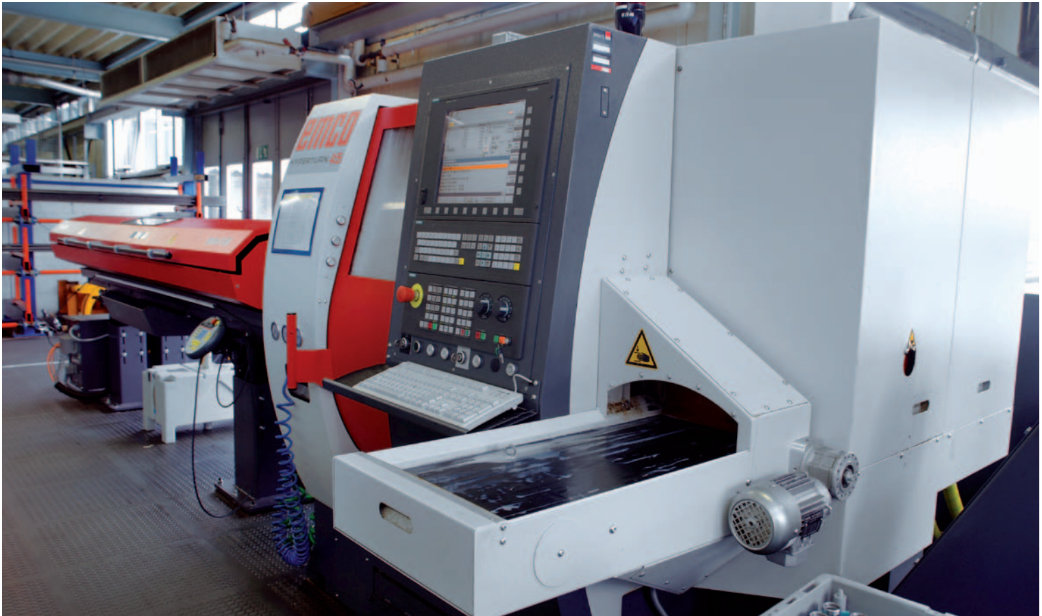
Hyperturn 45 equipped with Turbo 5-55: Fully automated bar loading for bars with a diameter of up to 65 mm, whilst the work pieces are finished via sub-spindle by means of the tools in the turret.
