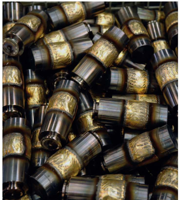
Three-part solenoid tubes – The example shows the brazed primary products, finished to precision parts with a Hyperturn 45 machine by drilling, turning and thread-cutting from both the outside and inside.
