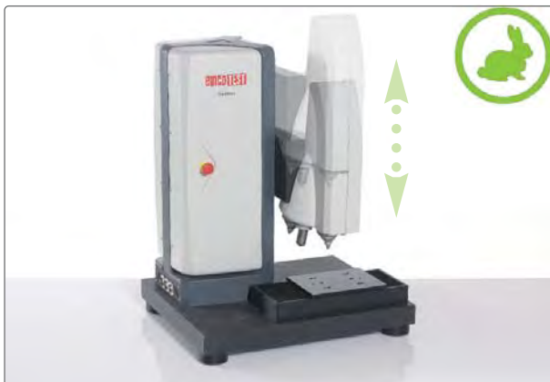
Patented height adjustment with rapid traverse
