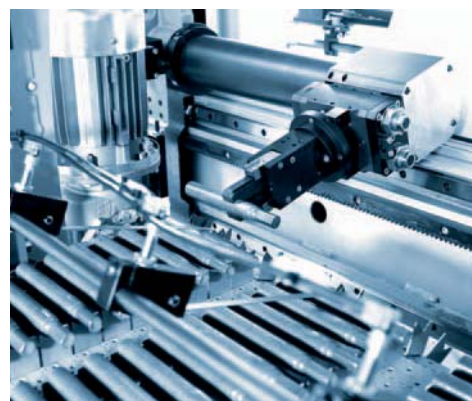
Timed conveyor system with V-supports for preformed shaft parts of various shapes.
