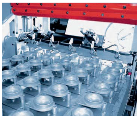
High-capacity timed conveyor system for correct directional loading of pre-formed blanks.
