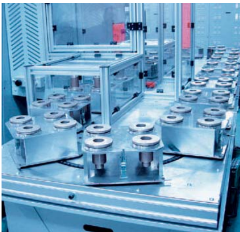
4-station pallet attachment for valve caps
