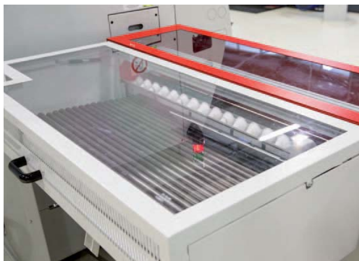
Material storage. The material storage surface with a length of 560 mm is arranged at the rear of the bar loader in a manner with no influence whatsoever on the space available. Depending on the diameter it is possible to store a different number of short bars.
