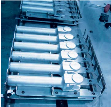
6-station pallet attachment for articulated brackets
