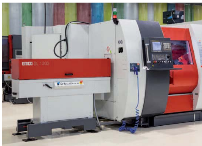
EMCO SL1200. Space-saving and cost-effective bar loading magazine. Operation and programming could not be easier. May also be used for loading single items through the lathe's main spindle.
