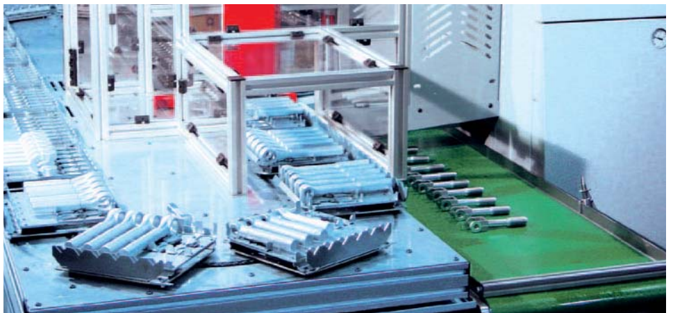
20-station pallet magazine with customer-specific pallets
