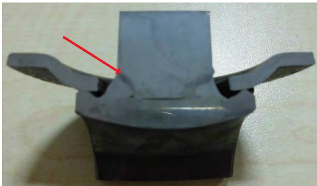
Grinded with SiC Paper
