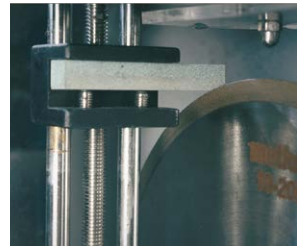
Blade dresser available for dressing even during cutting
